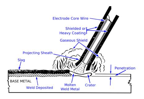
**Stick welding** (SMAW or Shielded Metal Arc Welding) is one of the most popular welding processes along with MIG and TIG. It's a simple procedure that is popular with outdoor welders due to it not being affected by wind – unlike MIG and TIG welding which uses gas cylinders.
